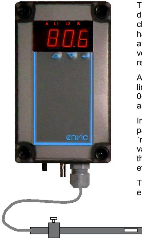
The DP-101S-AF is a surface mounting meter with a 4 digit numerical display intended for the measurement of air-velocity in air-conditioning, clean room, fume hood etc. applications. The measurement unit also has an area x air-velocity calculation function which allows the display and the output to be scaled in air-velocity measurements to give the flow volume. It is delivered with a built-in sensor and is pre-programmed ready for use.
